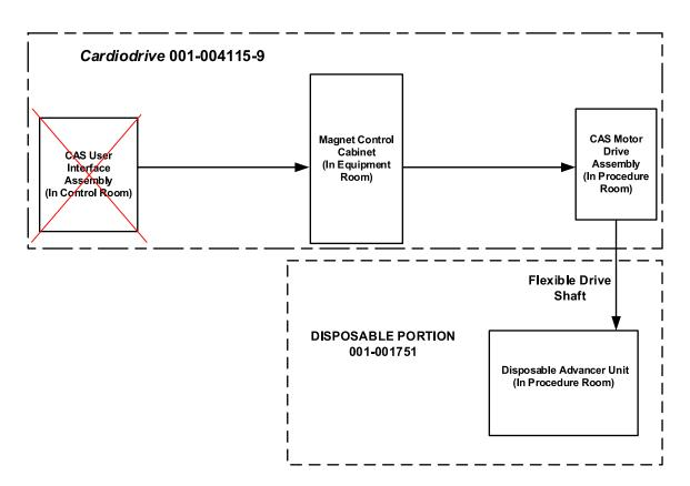
Figure 2. Cardiodrive interconnect diagram
