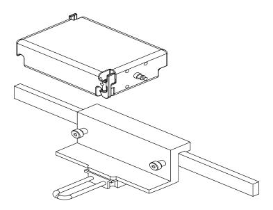
**Figure 3.** Motor Assembly mounting hardware installation
