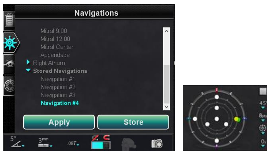
Figure 79. Store button is enabled ( left ) when Bullseye Targeting hits target ( right )
