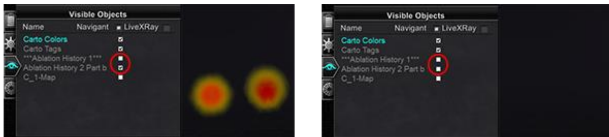
Figure 186. Encircled checkboxes show number of Ablation Histories displayed at right of each example: Left , Only “Ablation History 2 Part b”; Right , Neither Ablation History
