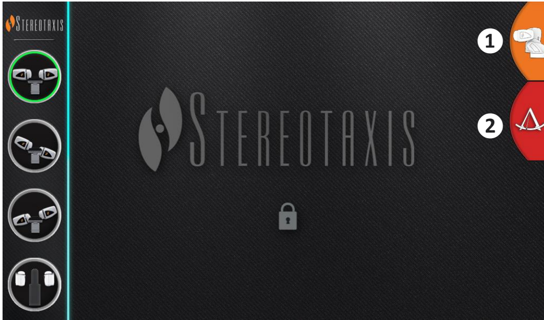
Figure 11. UTSC panel: Left , UTSC buttons; Right , (1) Enlarges and displays 4 more buttons in next screen ( Figure 12 ); (2) Links to Navigant screen.
