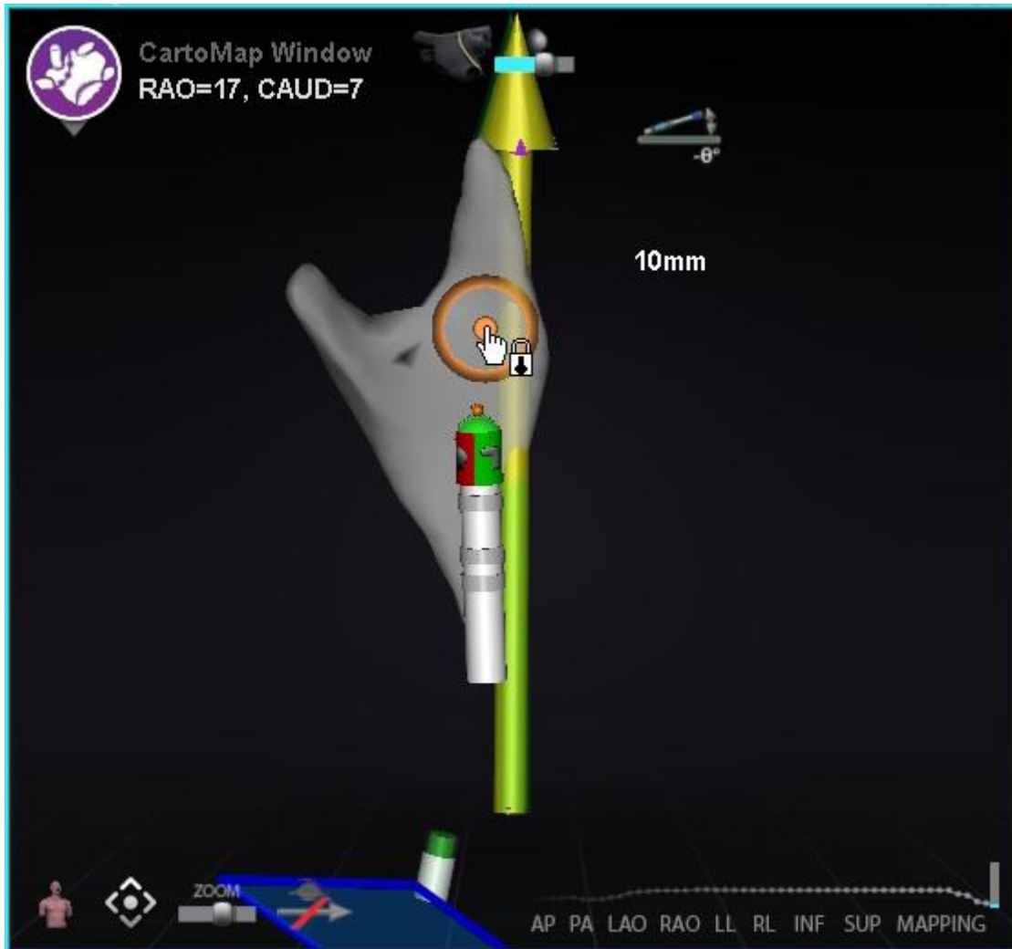
Figure 116. Target Lock (cursor's lock icon is showing with finger point at center of target)
