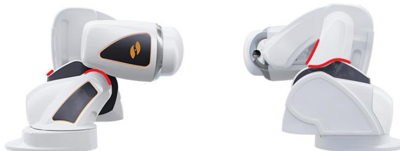
Figure 10. Red shading indicates pinch hazard areas ( left, Front; right, Back )
