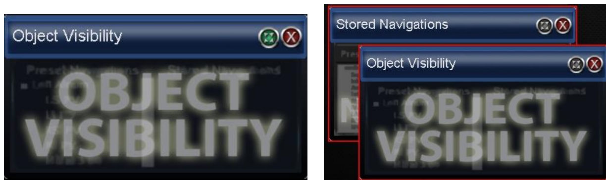
Figure 96. Left: Control panel with bright blue border because it is selected; Right: Two control panels with red borders because they overlap each other
