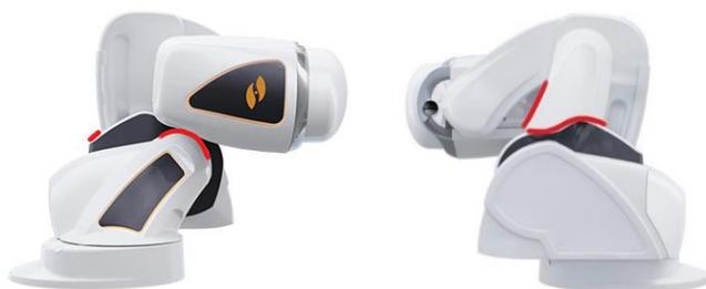
**Figure 10. Pinch hazard areas (red shading)**
