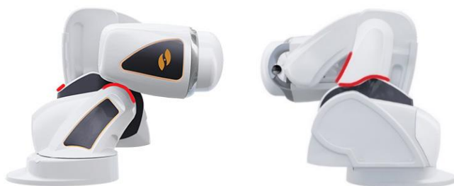
Figure 10. Pinch hazard areas (red shading)
