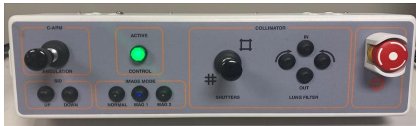
Figure 14. Model S Control Panel in Control Room and Procedure Room
