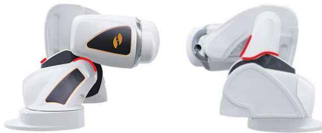
Figure 10. Pinch hazard areas (red shading)
