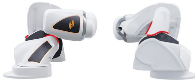
Figure 10. Pinch hazard areas (red shading)
