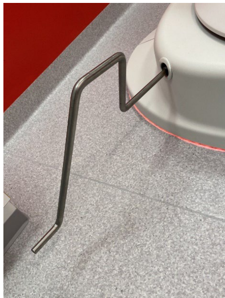
Figure 23. Hand crank bar inserted into access port
