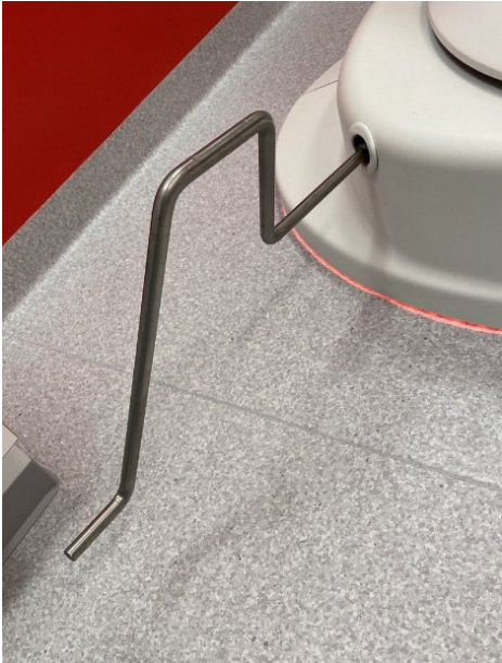
Figure 23. Hand crank bar inserted into access port
