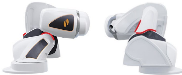
Figure 10. Pinch hazard areas (red shading)
