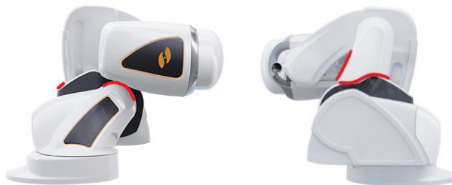
Figure 10. Pinch hazard areas (red shading)
