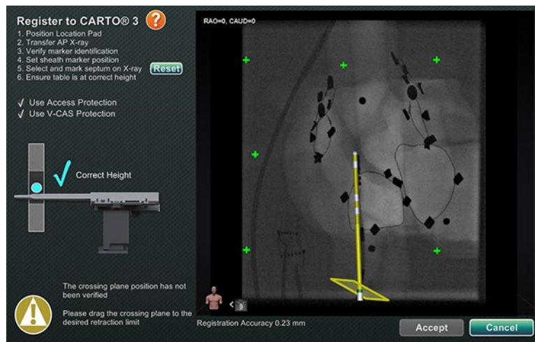
Figure 64. Crossing Plane Needs Adjustment
