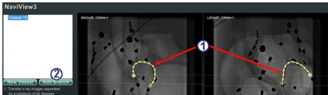
Figure 129. Adding branches – Start with matching trunks
