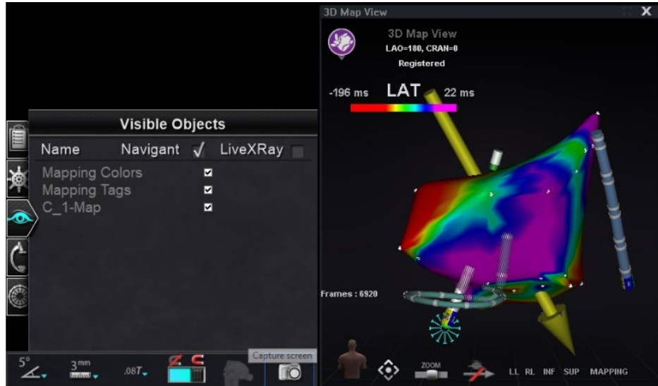
Figure 26. Mapping Colors and Mapping Tags
