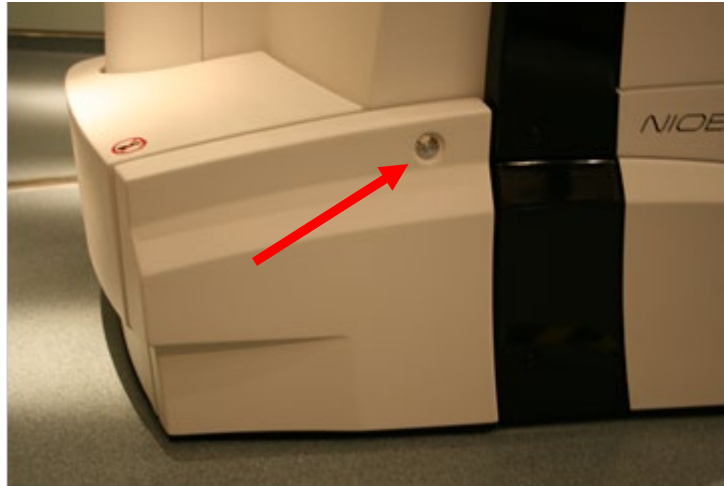
Figure 244. Niobe ES cover for emergency manual pod movement
