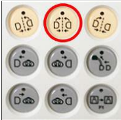
Figure 14. Navigate AP button is top-middle button on Tableside Controller (Philips/Model S colors displayed)
