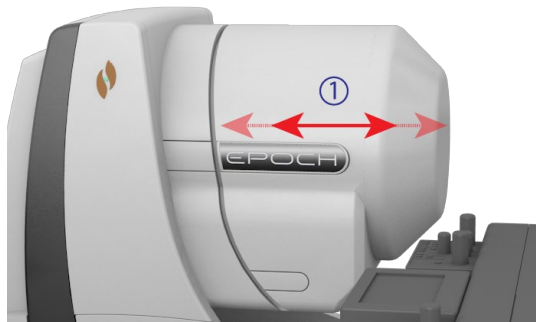
Figure 20. Niobe ES magnet cover moves toward and away from patient table (see guide below for numbered references)
