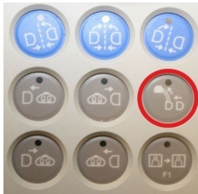
Figure 15. Stow button is on far right of second row of Tableside Controller (Siemens colors displayed)
