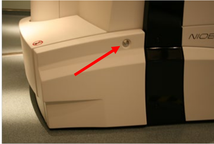
Figure 20. Niobe ES cover for emergency manual pod movement
