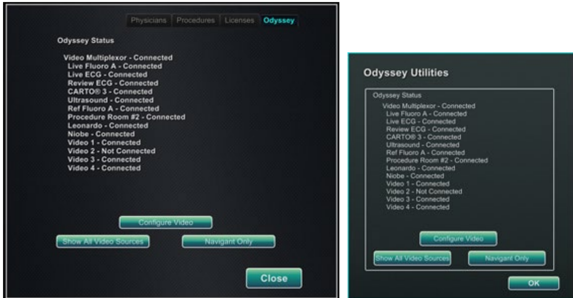
Figure 61. Odyssey utilities dialogs with connection statuses: Left, from start panel; right, from system options button
