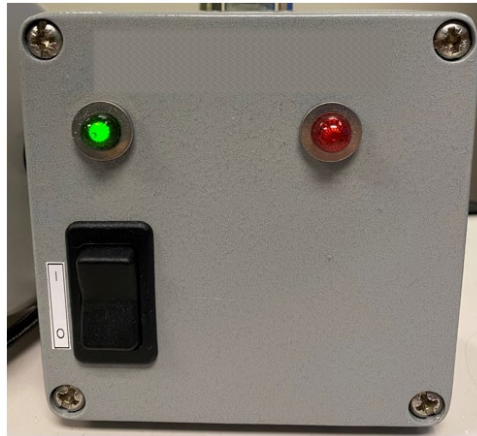
Figure 10. Remote System Power Box
