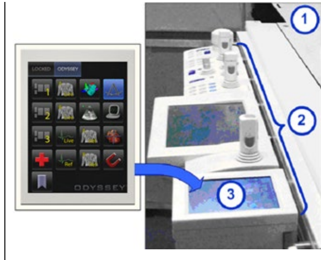
Figure 2. Tableside Controller on patient table accessory rail
