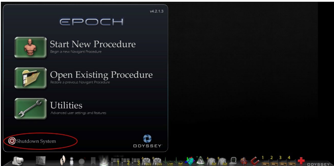
Figure 51: Start panel with Shutdown System button
